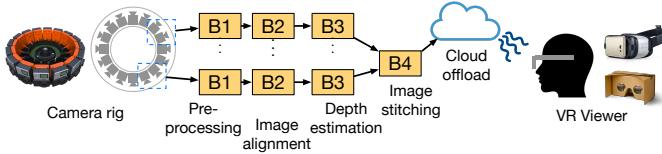
Fig. 10. 3D-360° virtual reality video generation, capture and viewing devices.
