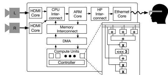
Fig. 13. VR accelerator architecture on a Xilinx Zynq SoC.
