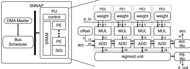
Fig. 3. NN microarchitecture and processing element details.
